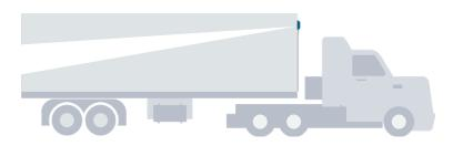
Place the tracker has high as possible on the asset to ensure good network coverage.
