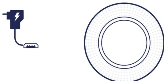
If your ethernet network supports Power Over Ethernet (PoE) the zone anchor draws power over the ethernet cable and no micro USB power connection is needed.
