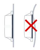
Make sure the mounting surface is flat and clean, for a strong and durable bond.
