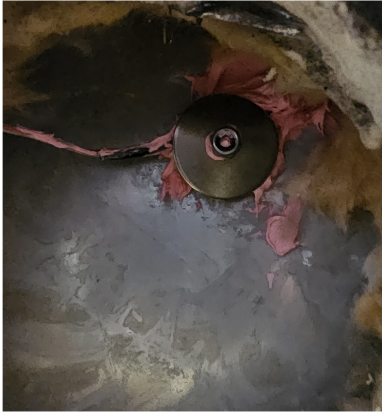
Mount the probe with thermal paste
