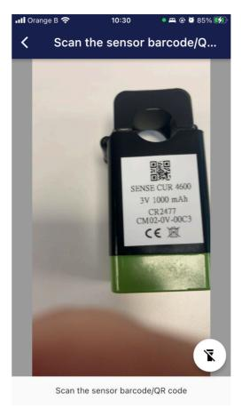
Scan the the QR code of the the sensor, the sensors slots will be automatically assigned
