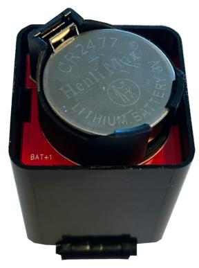
2. Place the battery with the - pole down
