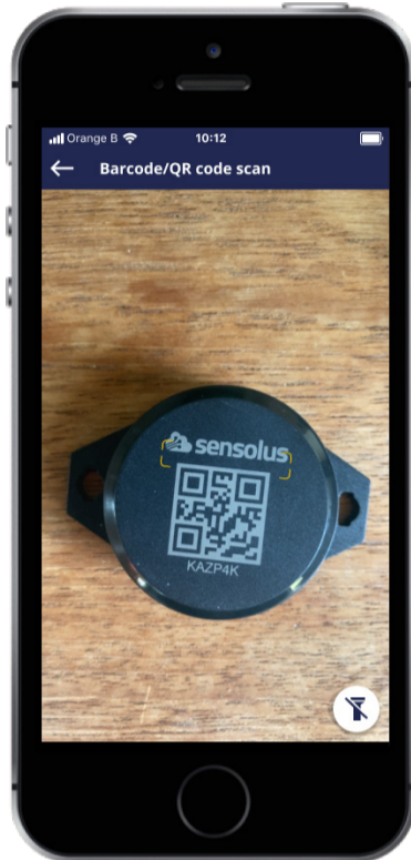
Scan the Barcode printed on the front of the BLE tracker.
