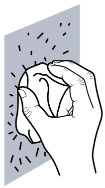
Clean the area on the asset where you want to add the tag and also the back side of the tag to get rid of any grease/oil.
