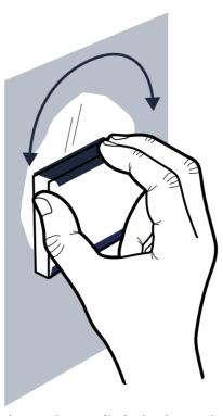
Sand both surfaces lightly for a few seconds to increase surface area.
