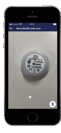
Scan the Barcode printed on the front of the BLE tracker.
