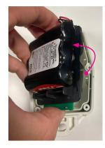
**Step 3** Take the module (Battery pack + battery holder + PCB) out of the casing.
