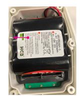
**Step 11** Place the module in the tracker. Use the alignment marks on the casing. Do not use force. There is only one way to put the module back in the tracker.
